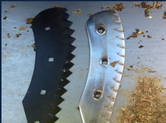
Figure 21 a), b) New and worn mixer wagon knives. Source: FeedWorks (2026).
