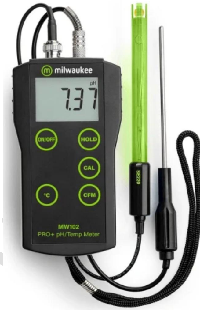
Figure 30 Example of a portable pH meter that can be purchased from a laboratory instrument supplier with calibration buffers (pH 4 and 7) and electrode storage solution for approximately $400-500. Source: Pacific Sensor Technologies (2026). Reproduced with permission.
