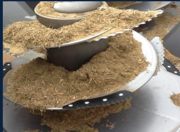
Figure 21 a), b) New and worn mixer wagon knives. Source: FeedWorks (2026).
