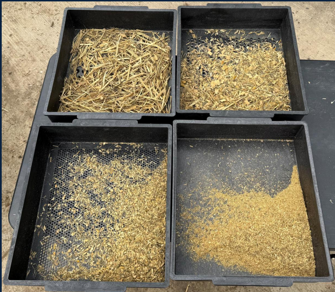
Figure 22 The three-sieve Penn State Particle Separator – regarded as the standard field method for assessing particle size distribution and the adequacy of physically effective fibre in TMR and PMR diets for dairy cattle. Source: Penn State University (2026). Reproduced with permission.
