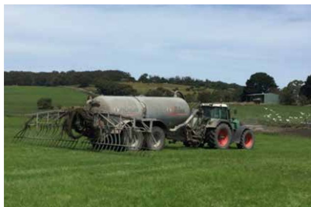
Figure 105. A trailing hose tanker spreading effluent from an agitated first pond
