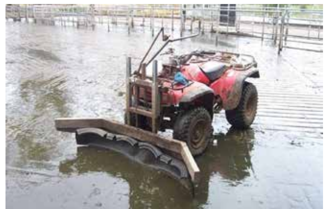
Figure 15. ATV mounted manure scraper
