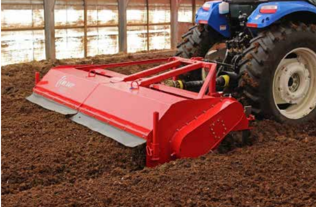
Figure 49. Roto-tillers may be used and are helpful to break up clumps of bedding material and maximize oxygen/air infiltration into the pack providing a uniform mix of material
