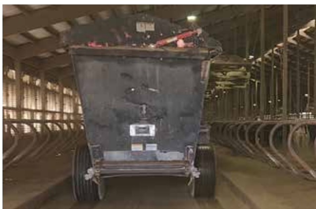
Figure 63. Machinery is used to add fresh bedding to stalls
