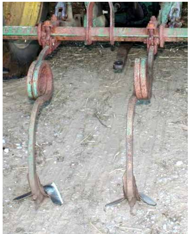
Figure 48. Sweeps or shovels may be added to tillage implement tines to provide more effective stirring. This is a cheap and effective addition to existing implements
