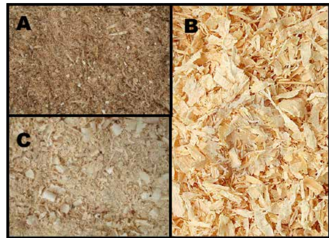
Figure 43. Sawdust from (A) sawn wood, (B) planed wood, (C) mixture
