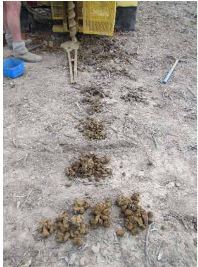
Figure 5. Layers of soil extracted from investigation using a drill rig
