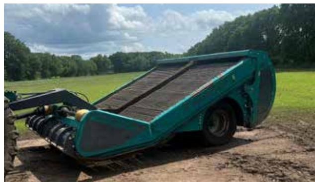
Machinery used for cleaning sand sheds
