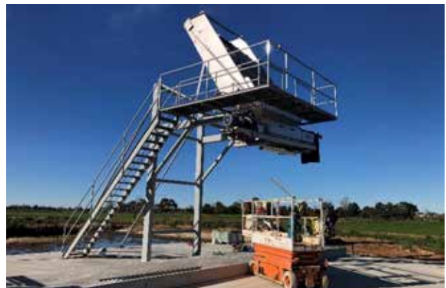
Figure 18. Mechanical stationary screen – screw press combination
