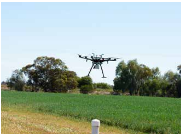
Figure 3. Developing a property image using drone technology with a phoenix Lidar sensor
