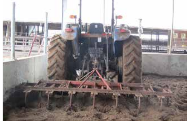
Figure 48. Sweeps or shovels may be added to tillage implement tines to provide more effective stirring. This is a cheap and effective addition to existing implements
